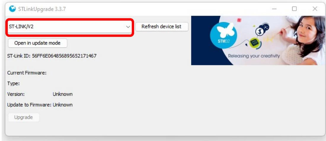
**Step 4-** Select **Open in update mode** in STlinkUpgrade window. After selection, current ST-LINK firmware details are fetched.
