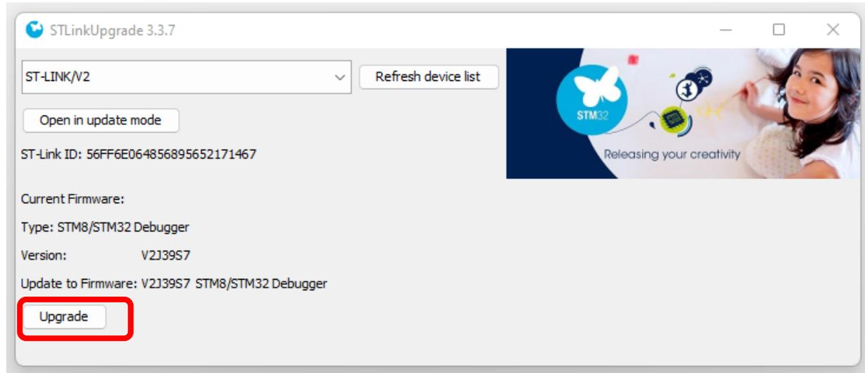
**Step 6-** After upgrade selection, upgradation process will be started and after successful completion Upgrade successful message will appear .
