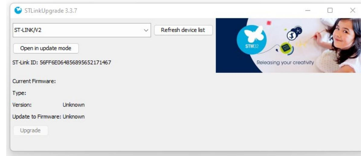
**Step 3-** STlinkUpgrade window will shows connected ST-LINK/V2 device.
